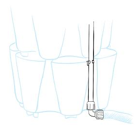
7. If you would like more space between your hose and your planter, use the tubing elbow in step 4 to create an "L" with the two pieces of tubing. Then attach the hose connector at the end of the second piece of tubing.
