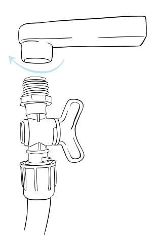
**4.** Connect the open end of the tube to the hose adapter. Similar to step 2, open the collar by turning counter-clockwise and work the tube onto the adapter. Once the tube is on, turn the collar clockwise to tighten.
